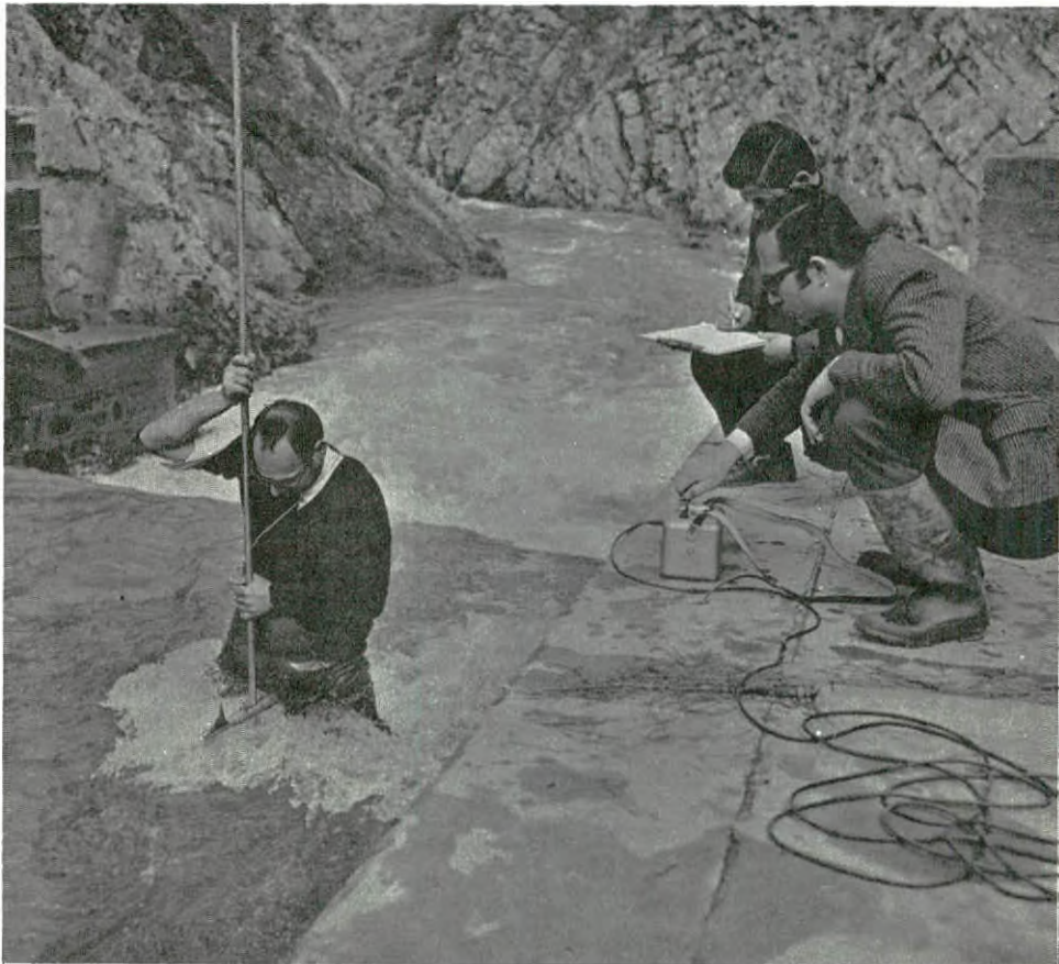
Wading across the river for Flood-discharge measurement by current meter at Peristerona gauging station
