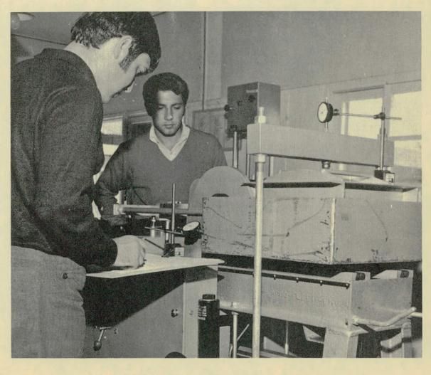
Large shear box test machine used for finding the shear strengh of cohesionless soils and crushed rock.
