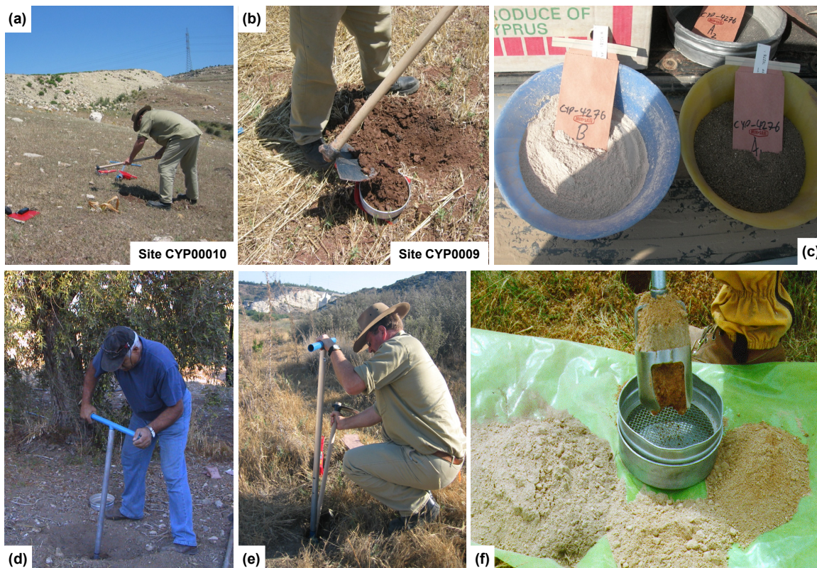
Figure 2.10 (a) and (b) stripping of recent organic deposits from the surface and excavation of upper 25 cm using pick or spade; (c) sieved materials (~400g); (d and e) excavation by auger and packing soil down in auger with cleaned pick handle (f) Jarrett-type steel augers with 20 cm steel flights and W-tipped cutting edges. Intermediate 20-cm intervals between the top and sub sample were also examined.
