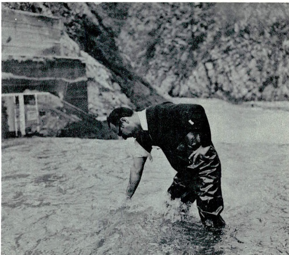
Taking sample of Water from Peristerona river for chemical and Suspended Sediment Analysis
