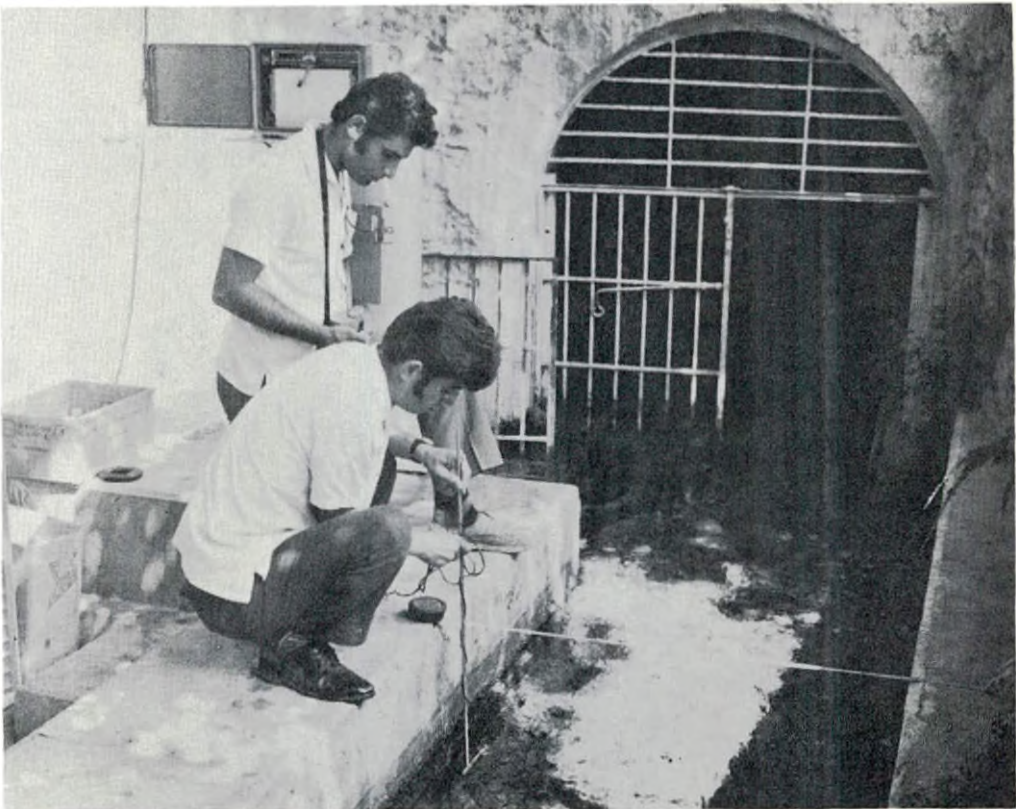
Measuring the Water velocity and flow with a current meter at the outlet of Kephlovrysos Spring at Kythrea.
