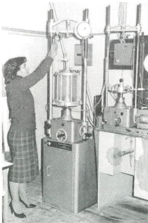
Large dia. Triaxial test being carried out at the WDD Soil Mechanics Laboratory for determining shear strength of materials up to 20 mm max particles size. WDD Photo 75 EN-O (2.10.81).
