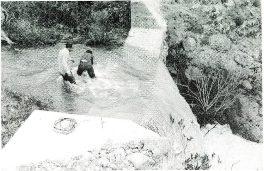
Calibration of Akapnou river gauging weir station at Melini by means of current meter measurements. WDD Photo 82 EN-25 (13.2.81)
