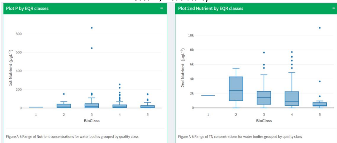
Figure 3-4 Macroinvertebrates, STAR-RM4. Plots TP (1 st Nutrient) & TN (2 nd nutrient) by EQR (High=5, Good=4, Moderate=3, Poor=2, Bad=1)
