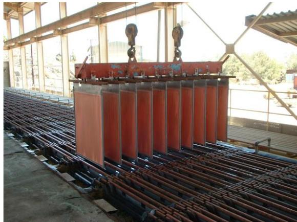
Figure 96 Finished cathodes being removed from cell.
